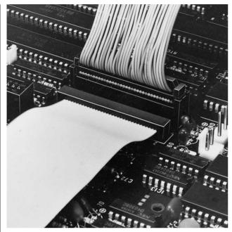
The RC connector is a board-in type insulation displacement connector for 1.27mm pitch ribbon cables. The number of positions match the RA disconnectable connector series so that they can be used as a pair on opposite ends of a harness.
