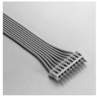
This is a 2.5mm pitch insulation displacement connector that is soldered directly onto printed circuit boards, with a mounting height of 7.1mm and with a width of 4.1mm. The DB connectors can be used by themselves or in combination with NR or HR connectors.
