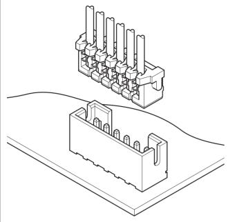
The KR connector features a mounting height as low as 6.9mm and a thickness as thin as 4.8mm (for top entry type). It is suitable for interconnection of a wide range of electronic equipment such as VCRs, video cameras, car stereo systems and communication equipment.
