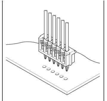
Measuring 2.0mm in pitch, 5.0mm in mounting height, and 4.0mm in thickness, this board-in connector is useful in miniaturizing the connections of small electronic products, such as VCRs, cameras, stereo systems, and car radios. This connector can be used by itself or in combination with the DR connector.
