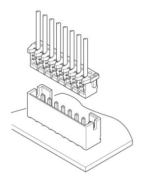
Multi-harness of CK connector (2.0mm) and CZ connector (1.5mm) combination has been realized. The in-line type IDC features low profile design with 6.9mm mounting height and 4.8mm thickness (top entry type).
