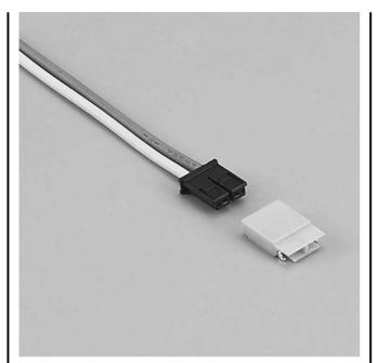
Low profile connector with high withstanding voltage, designed for connecting liquid crystal display backlight lamps to their starters. The BHL connector is 2.8mm thick, so the mounting height is only 3.0mm.
