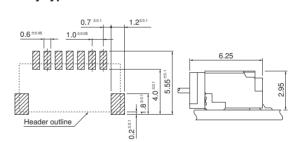
Note: 1. Tolerances are non-cumulative: ±0.05mm for all centers. 2. The dimensions above should serve as a guideline. Contact JST for details.
