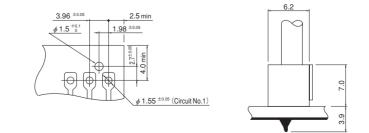
Note: 1. Tolerances are non-cumulative: ±0.05mm for all centers. For connectors with 5 or more circuits the hole dimensions will differ from the above values. Contact JST for details.
