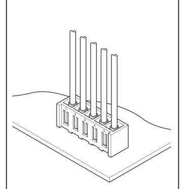
The SDN connector is a 3.96mm pitch board-in crimp style connector capable of connecting a wide variety of circuits including signal and power supply circuits. The connector features a slim, low-profile design. In addition, it has an exclusive lance construction to reduce insertion force, thus substantially improving the working efficiency in mounting the contact.
