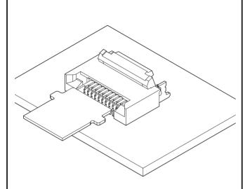
This is 2.0mm height connector with the double-sided contact for FPC. As FPC with protrusions is used for this FHH connector, prevention of incomplete insertion and misinsertion are realized and connection reliability is improved.
