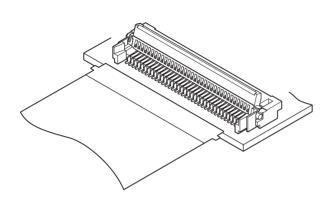
A substantial size for the 0.3mm pitch connector ensures easy handling. Moreover, since this connector accepts a FPC with protrusion providing secure as well as foolproof mating at the customers production line.
