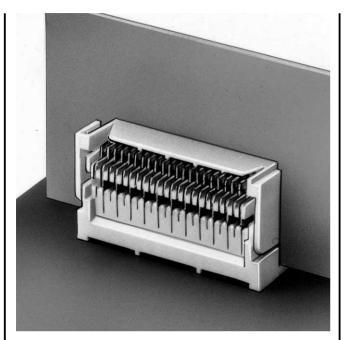
Hinge type board to board connectors which allow mated PCB's to move 90° in respect to one another while electricity is turned on. The hinge compensates for slight misalignments between circuit boards to assure a secure connection even if the boards are laterally out of line up to 0.5mm. Header leads are staggered for easy board design.
