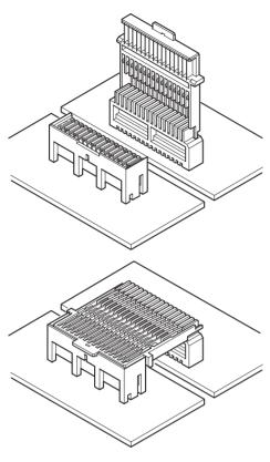
The 1.5FJ connector is a 1.5mm pitch board-to-board connector. Its plug consists of a unique flexible hinge that absorbs circuit board misalignment. Board-to-board connection requires less labor and is more reliable because the connection can be made without the use of harnesses after the printed circuit boards are installed in their enclosures.
