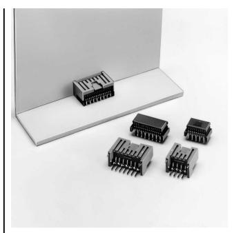
Self-supporting style board to board connectors. Both plugs and receptacles are supplied radial-tape mounted (conforming to JIS C 0805 tape specification), which can be mounted by versatile, radial component pick and place machines. Automatic mounting is possible up to 15 circuits.
