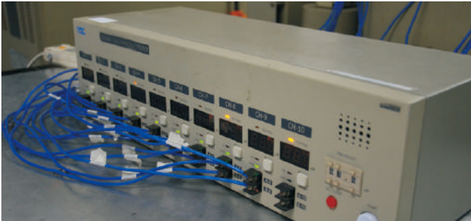
Electric Current Break Test Equipment
