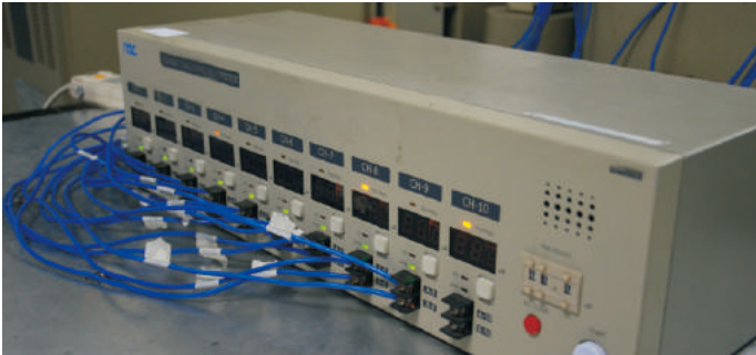
Electric Current Break Test Equipment
