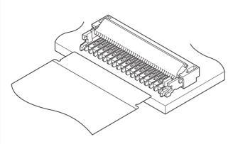
0.2mm pitch FVXS connector for FPC has been developed for small portable equipment for which low profile and miniaturization are required. Positioning of FPC is easily conducted by inserting FPC into connector until its shoulder touches to the transverse U-shape groove.
